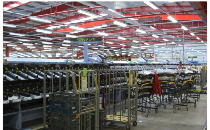
iLSM sorter trays and speed indicator
